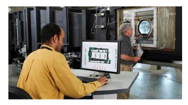
Our facility includes one of the most capable wind tunnels in the world — blasting ice particles at Mach 0.9 and providing temperatures down to -90°F (-67°C) and altitude up to 50,000 feet (15,420 meters).
