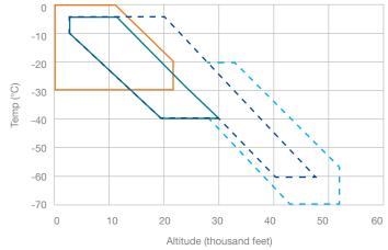
Part 25 App. C (Continuous Maximum) Supercooled Water Droplets (SD)
