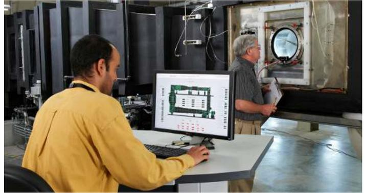
**Our facility includes one of the most capable wind tunnels in the world – blasting ice particles at Mach 0.9 and providing temperatures down to -90°F (-67°C) and altitude up to 50,000 feet (15,420 meters).**
